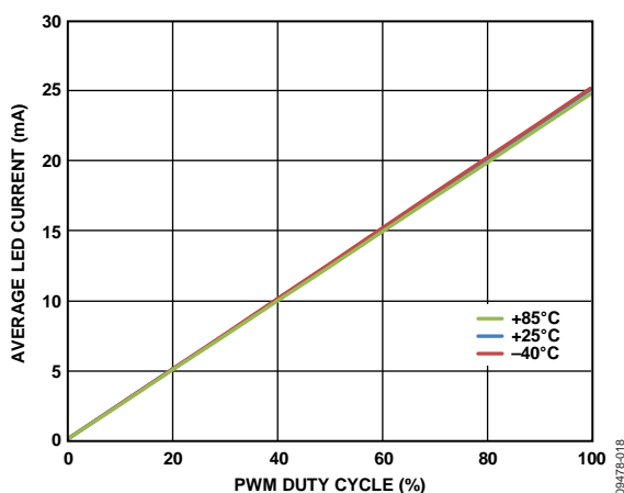
Figure 18. Typical Average I_{OUT} vs. PWM Duty ( f_{PWM} = 300\text{ Hz} )
